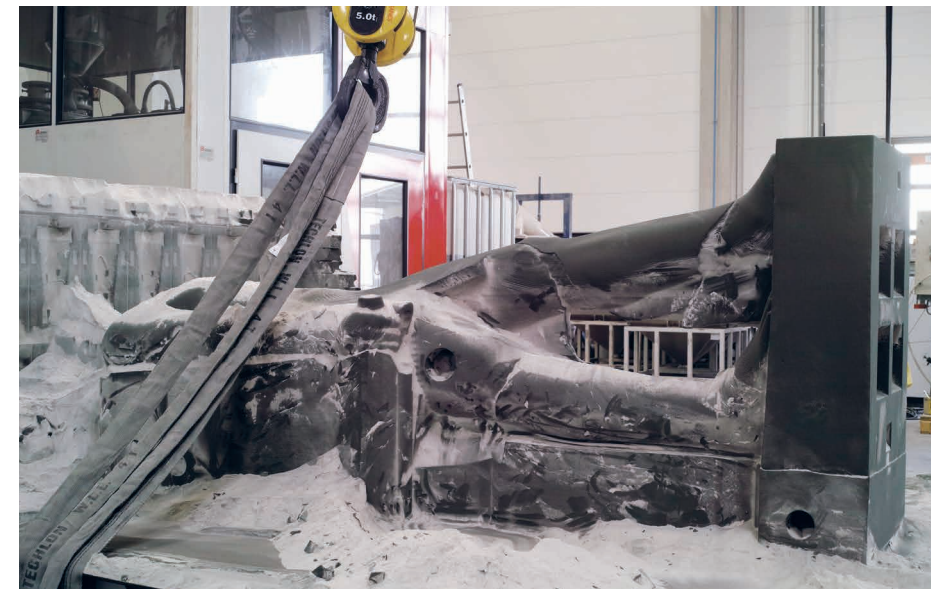
3D sand-printing of Taharqa at Voxeljet, Friedberg/Germany, July 2014.
